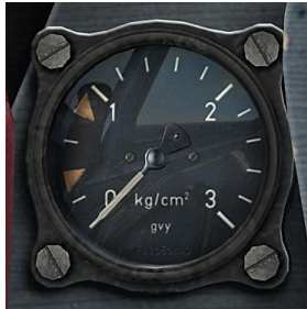
Figure 31: Water/Methanol Pressure Gauge
