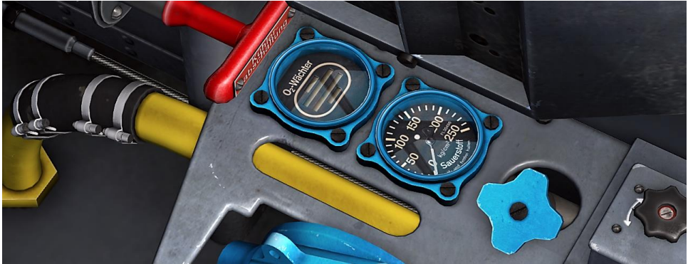
Figure 46: Oxygen Flow Indicator and Pressure Gauge
