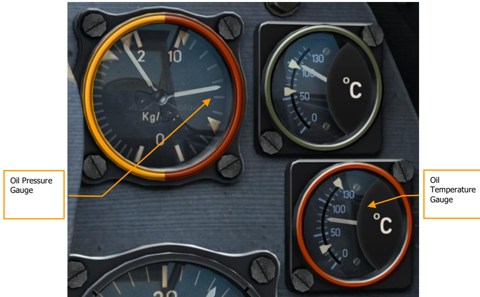
Figure 42: Oil Pressure (right) and Oil Temperature Gauges
