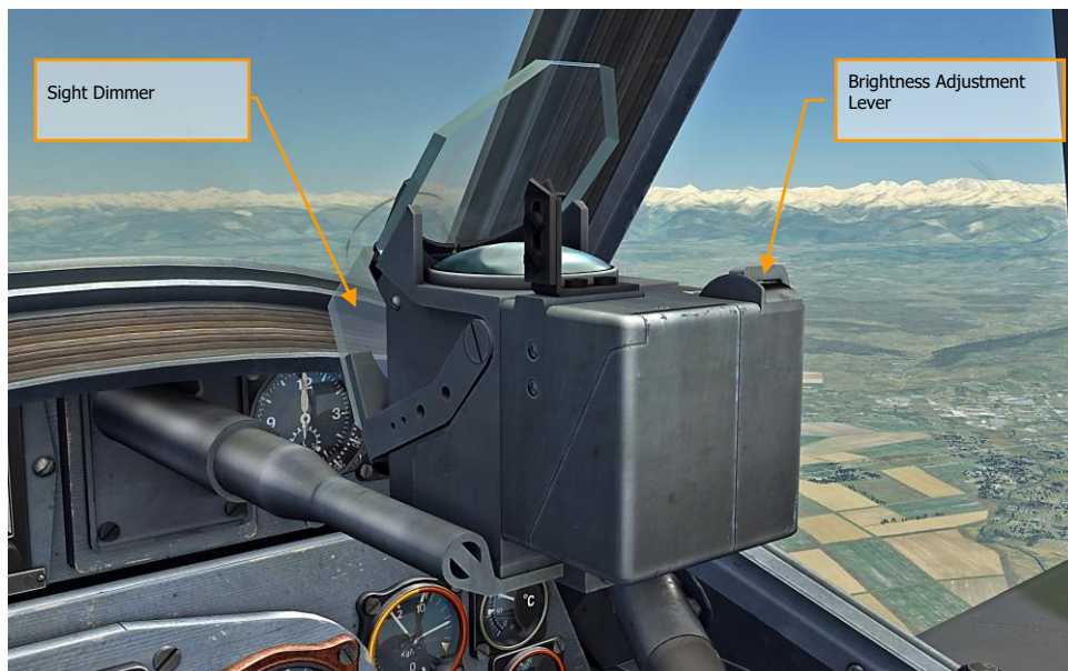
Figure 61: Revi 16B Gunsight in unfolded combat position
