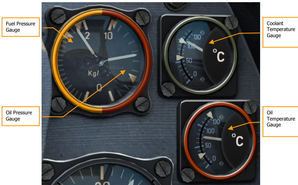
Figure 78: Fuel and Oil Pressure Gauge, Coolant and Oil Temperature Gauges
