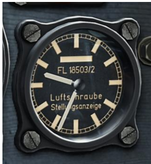
Figure 80: Prop Pitch Indicator in 9:34 Position
