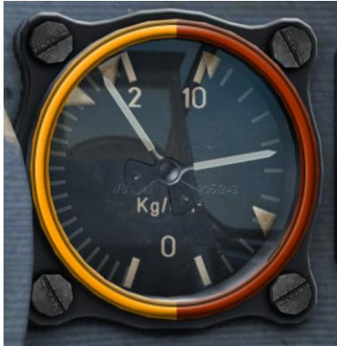
Figure 37: Fuel Pressure (left side) Gauge
