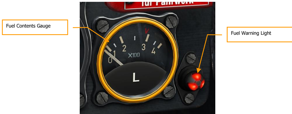
Figure 81: Fuel Contents Gauge and Fuel Warning Light
