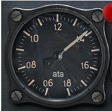
Figure 29: Supercharger Pressure Gauge
