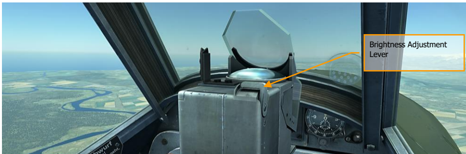
Figure 62: Gunsight's Brightness Adjustment Lever
