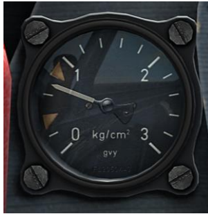
Figure 68: Water/Methanol Pressure Gauge
