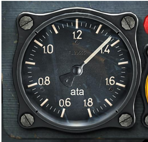
Figure 83: Supercharger Pressure Gauge
